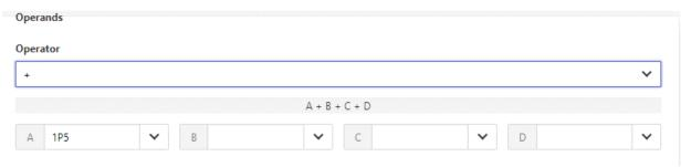
The drop-down list below shows the different operations that can be performed on the operands. Note that the number of operands will automatically adjust from 1 to 4, depending on the nature of the operation selected. The information window, located just above the operands, shows the actual equation with the relation of the different parameters.
