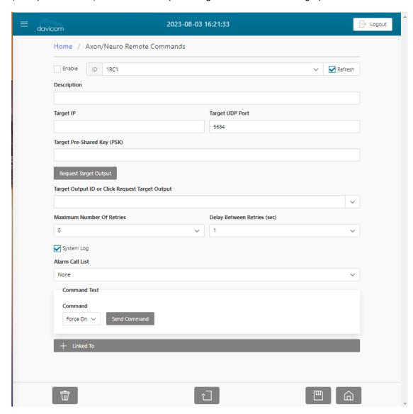
A **Send Command** test button is also available to validate operation during setup.
