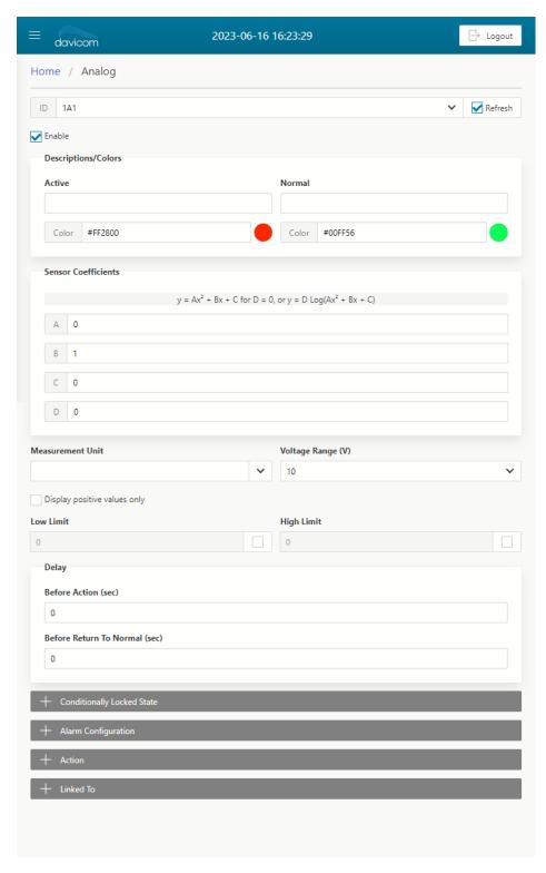
The A, B and C parameters allow sensor linearity, gain and offset to be fine-tuned, respectively. The corresponding equation is shown in the View window. The D parameter is used for logarithms as also shown in the equation.
