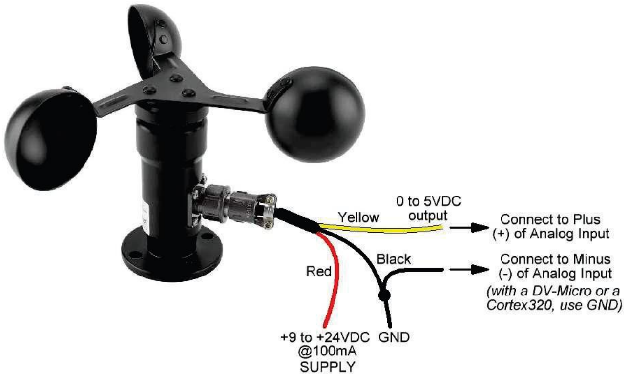
Figure 1. Wiring instructions for 0-5 Volts output.
